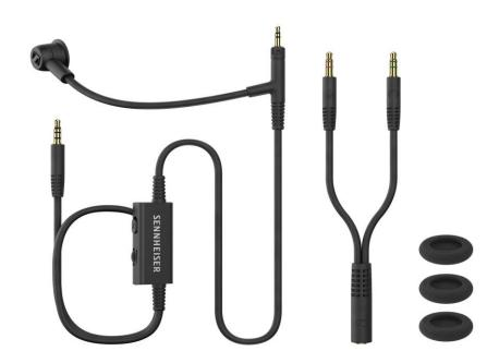
To ensure flexibility across a vast range of devices, the HD 500 BAM uses a 4-pole 3.5mm plug with CTIA wiring, and an in-line volume control with mic mute switch along its 1.5 meter / 5 foot cable, a trio of windscreens and a Y-adapter for PC soundcards with discrete microphone and headphone connections are included.
